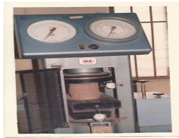
Plate 2: Compression machine armed with dial gauges
